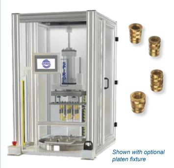
The SPIROL Model PH Heat Insert Driver provides an accurate and consistent method to simultaneously install multiple Inserts or Compression Limiters at multiple elevations. Simultaneous installation dramatically increases productivity and simplifies the number of manufacturing steps to complete an assembly. Additionally, the platen head and fixture can be easily changed to accommodate quick change-over to different assemblies associated with new production runs.
