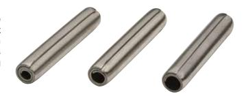
The **duty** (or material) thickness of the coiled pin can be varied to provide the optimum combination of strength and flexibility. The lighter duty pins require less insertion force, thus reduces the cost of the automation equipment because a smaller cylinder and/or machine can be used.
