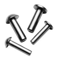
order utilise to traditional automating methods, headed parts should be able to hang by the head. A good rule of thumb is that there should be a minimum of a 20% differential between the head and body diameter order to provide enough distinction allow for orienting and
