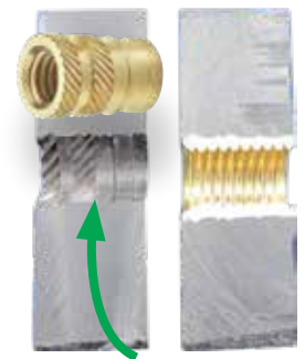
Figure 2. Proper Plastic Flow
