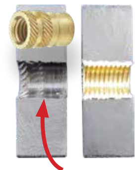
Figure 3. Improper Plastic Flow
