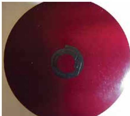
Photograph of a mounted and polished coiled spring pin. This pin is now prepared for microhardness inspection.
