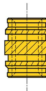
Finally for best performance, it is essential that the Insert is installed axially square to the hole. This can be facilitated with tapering the Insert or by providing a pilot. Pilots need to be of sufficient length and have a plain, unknurled diameter the same size or slightly smaller than the hole.
