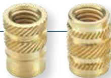
**Series 19 and 29** are designed for straight holes using standard core pins. The same hole diameter applies to all Inserts within these Series. Seating and installation are facilitated with a pilot and a tapered knurl and groove design. The Series 29 is symmetrical to eliminate the need for orientation.
