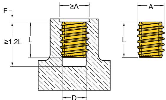
Counterbores are also recommended for Headed Inserts so that the top of the Insert will be flush with the surface of the plastic after installation. The diameter of the counterbore should be 0.5mm (.02") to 1.3 mm (.05") larger than the head diameter of the Insert. The minimum depth of the counterbore should be specified as the thickness of the head. Insert heads are sometimes left above flush to reduce jack-out or improve match-up with the mating component.
