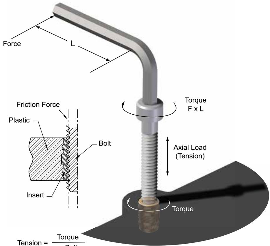
$$\text{Tension} = \frac{\text{Torque}}{\mu \times \text{Bolt } \phi}$$
