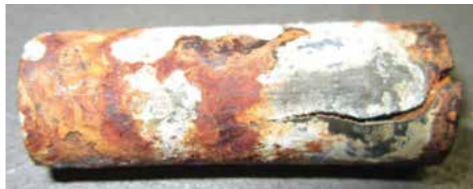
Figure 2: This Coiled Pin was finished with a light duty zinc plating and subsequent chromate dip. The finish was rated for 48 hours to 'red' corrosion protection. Leaving this item in salt spray for 200 hours has resulted in significant red rust though some zinc and white corrosion remain. Where zinc is present on the surface, the part remains free of red rust despite the severity of attack in adjacent areas.
