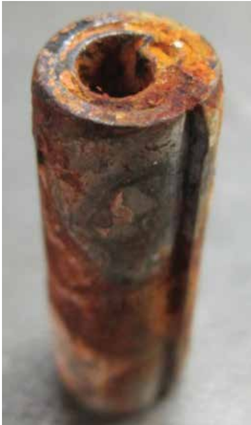
Figure 3: This photograph demonstrates the basic geometry of a Coiled Pin – it consists of a number of metal wraps. Platings will not penetrate between the wraps and dip coatings, though capable of covering the interior, will remain ineffective between the pin's wraps.
