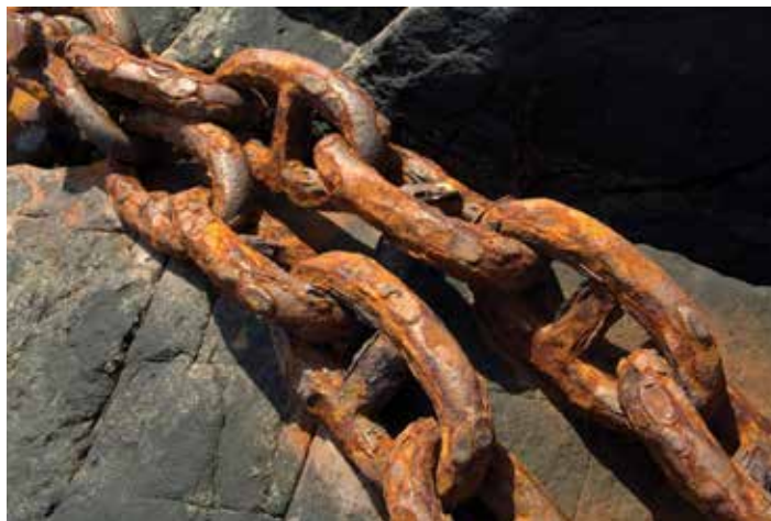
Figure 1. Rusting chain demonstrates material loss due to rust or general attack.
