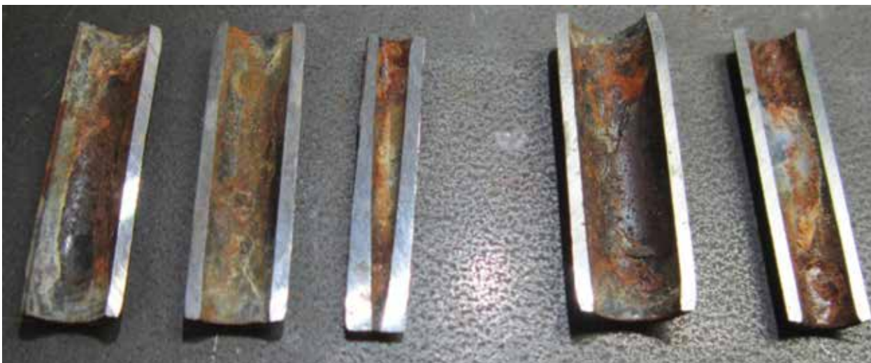
Figure 4: To demonstrate attack between the Coiled Pin's coils (or wraps) of steel, the photograph below was taken after cross-sectioning the pin shown in Figure 3.
