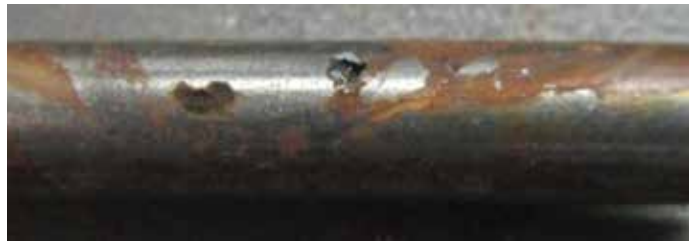
Figure 7: Pitting with related staining on 420 stainless Slotted Pin.
