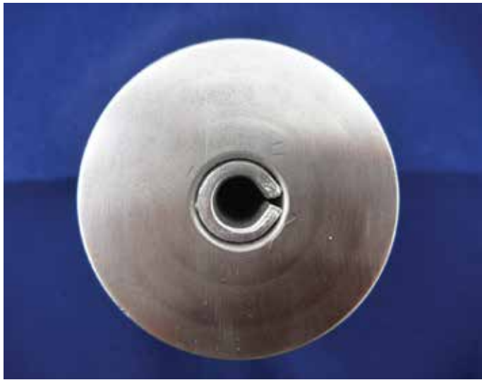
Figure 5: Slotted Pin installed in a nominal recommended hole. Notice the gap is virtually closed along the inside diameter of the pin.
