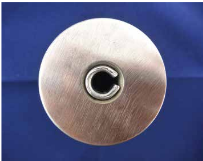
Figure 6: Slotted Pin installed in a oversized hole.
