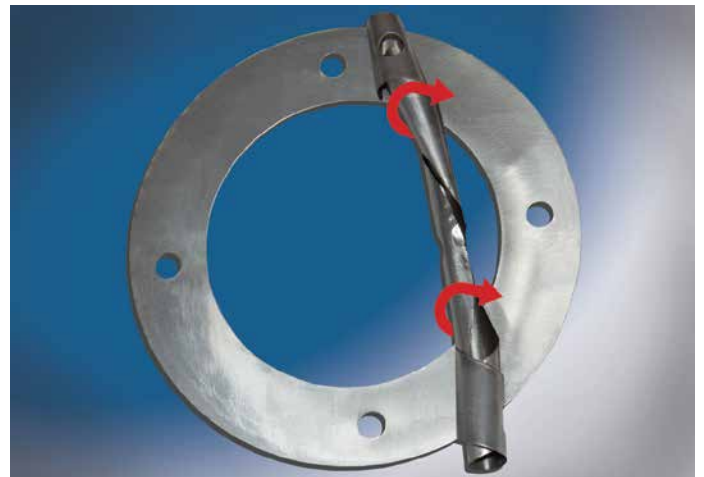
Surface Bonded Laminated Shims unwanted layer deformation
