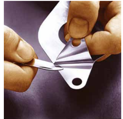
Laminated shims can be peeled down, layer by layer, until they are the proper thickness.
